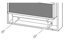
Figure 17 - Installing Bottom Mounting Screws
